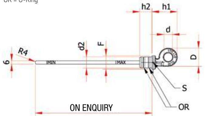
Push-fit dipstick with eye-handle, ensuring high mechanical resistance at both low and high temperatures, dimensional stability and shocks resistance.
