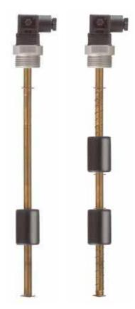
Level switch particularly suitable for hydraulics, lubrication plant, water treatment, industrial vehicles, fluid stocking, cleaning machines and equipment. The hermetically sealed reed switch housed inside the stem is actuated by a magnetic field created by a magnet equipped float. As the float rises and lowers with liquid level, the magnetic field passing the switch in the stem causes the switch to either open or close. Executions specifically approved R.I.N.A.
