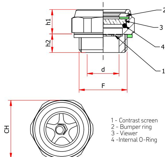
Threaded hex-head oil level indicator for screw compressors, gearboxes or any others applications where high pressure and mechanical resistance are required. Internal contrast screen in aluminum helps the control of the level inside the tank.
