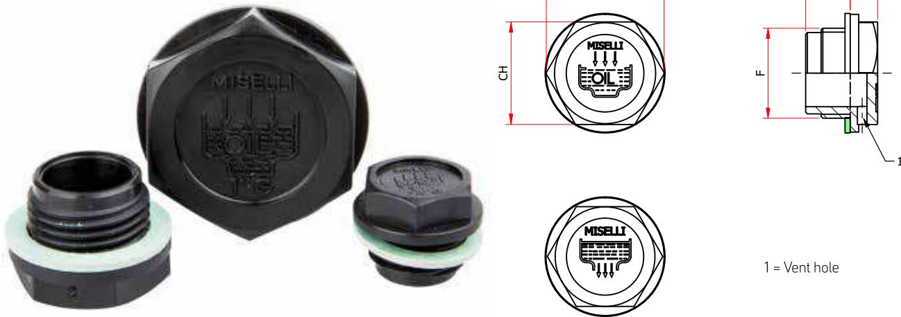
Threaded hex head oil plug ensuring high mechanical resistance at both low and high temperature, dimensional stability and shock resistance. TCN and TCNS style have the "fill" graphic symbol and the word OIL moulded on the top. TSN has a graphic symbol of drain moulded on the top.
