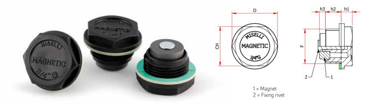
Threaded hex head oil plug that can be fitted on the bottom of the transmission or tank, to be used as drain plug; the magnet attract ferrous metal parts, preventing damage to gears and others moving components.
