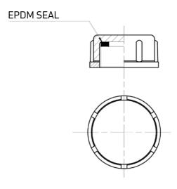
Blanking cap with internal thread designed for plastic tanks.
