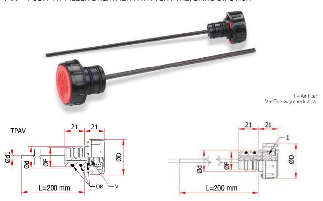
Filler breather, with easy grip vertical ribs, ensuring high mechanical resistance at both low and high temperatures, dimensional stability and shocks resistance. Push fit mounting into drilled hole (refer to corresponding sizes shown in the table below) tolerance  $\pm$  0,1 mm with 1/45° chamfer.
