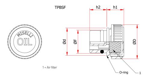
Knurled "low-profile" filler plug, applied where overhead space is limited. Push-fit mounting into drilled hole (refer to corresponding sizes shown in the table below) tolerance  $\pm$  0,1 mm with 1/45° chamfer.
