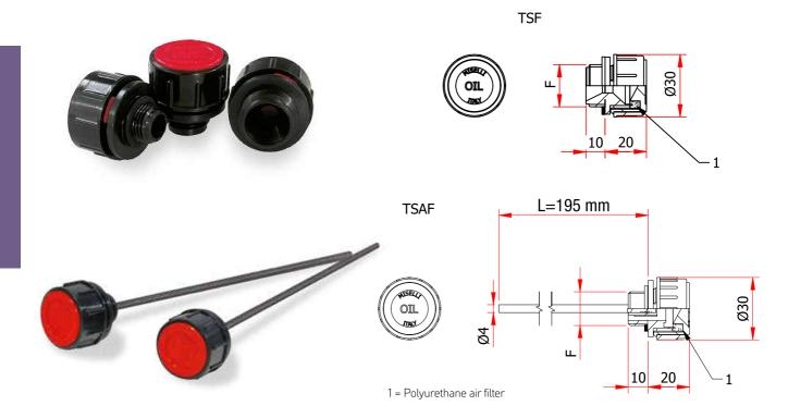
Threaded filler breather, cylindrical head 30 mm ø, with easy grip vertical ribs, ensuring high mechanical resistance at both low and high temperatures, dimensional stability and shocks resistance.
