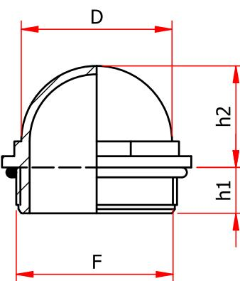
Dome shaped transparent level glass, enabling oil level to be read from any angle. This product is utilized on trucks/tankers and large reservoir containing liquids, especially in agricultural machinery.
