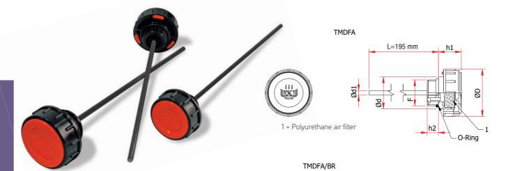
Threaded filler breather, cylindrical head, with easy grip vertical ribs, ensuring high mechanical resistance at both low and high temperatures, dimensional stability and shocks resistance. It allows air passage at high volume, through the vents located on the bottom of the head; recommended to be used in systems where frequent oil level changes take place in short amount of time, allowing the air to enter and leave the system, without any unwanted air pressure increase or decrease.
